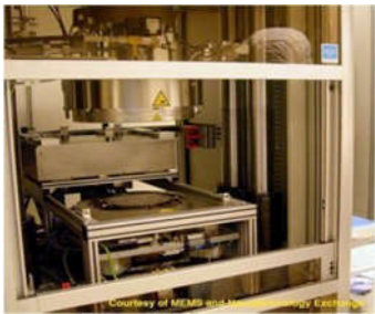
Fig 19: Photograph of a hot embossing platform during use. (Courtesy of the MNX at CNRI).
