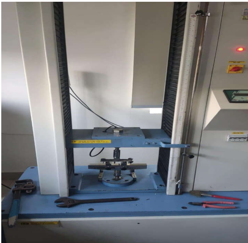
Figure2: 3-Point Bending machine Sample loaded condition for Flexural testing
