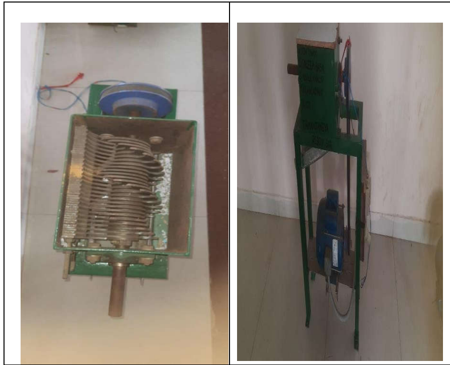
Figure 2: Sectional Views of Single-Shaft Shredder Machine
