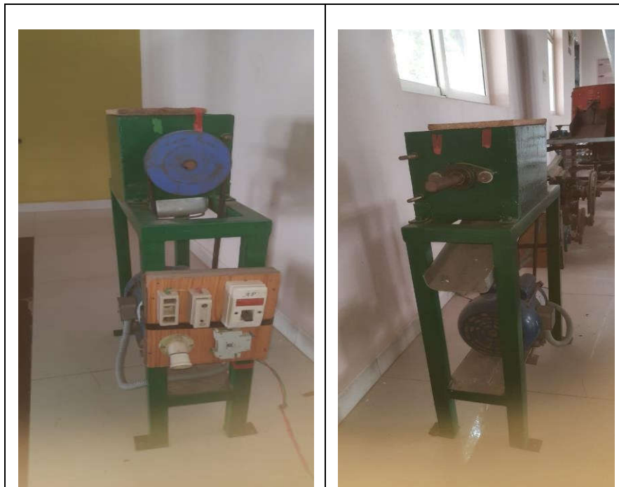
Figure 1: Sectional Views of Single-Shaft Shredder Machine
